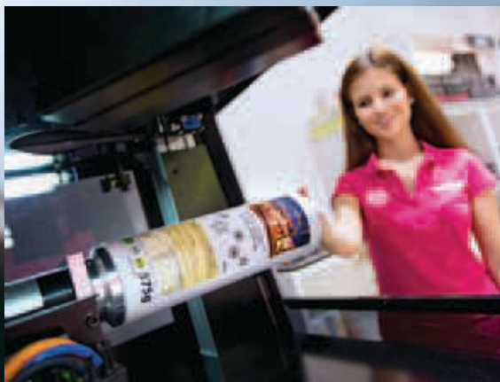
The muesli packaging is clamped in the Jetmaster Dimension 250 ready for printing. Customers can watch the printing process through the window.
