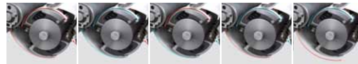
Three drum perfecting device in action: Sheet-stretching rotary suckers tighten the trailing edge of the paper before the patented pincer grippers pass the sheet along to the next impression cylinder. This design guarantees true-to-register sheet reversal and a controlled transfer to the next printing unit with a single gripper closure.
