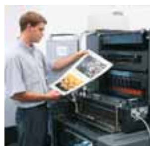
With the help of the Laco coating unit, the Printmaster PM 52 and the Speedmaster SM 52 can now also finish inline.
