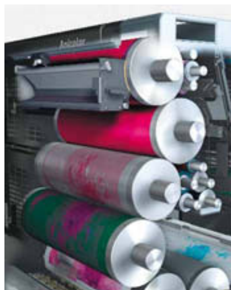
View of the Anicolor technology on the Speedmaster SM 52.
