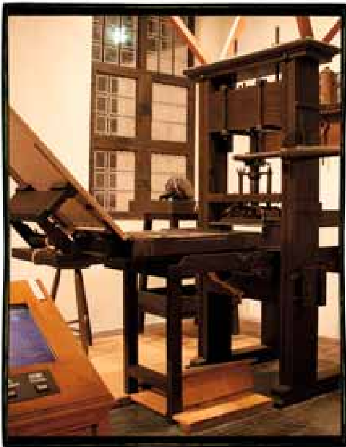
Replica of a wooden Gutenberg press from the 15 th century.
