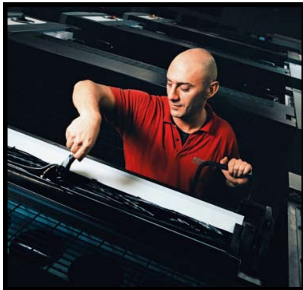
Extra large format: Printing Assistant Riccardo Ferrarese with a printing plate for the Speedmaster XL 162, which is 52.6 x 64.2 inches (1,335 x 1,630 mm). He fills an ink fountain on the new printing press.
