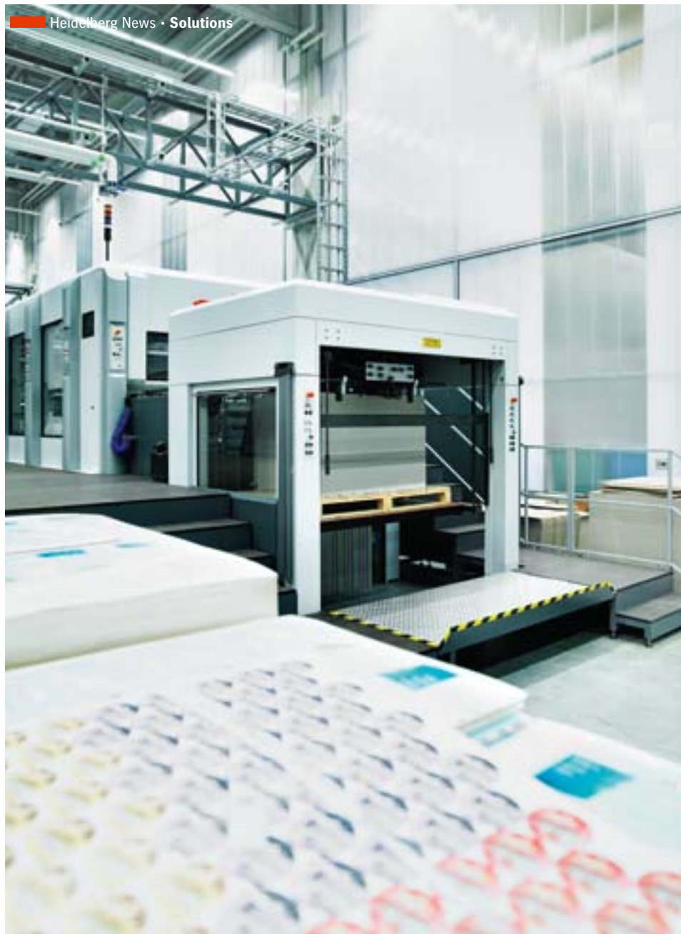
Ideal match for extra large format die-cutting: a Dymatrix 142 CSB.
