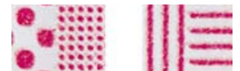
Slur (top) and ghosting (bottom), for example due to the wrong packing height, insufficient processing and too much pressure.
