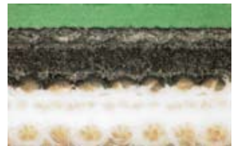
Cross-section of a blanket (Source: I.M.C GmbH).
