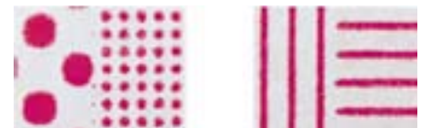
Good print image thanks to intact blanket.
