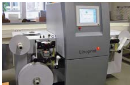
Drop on Demand – the first DriveLine digital printers from Linoprint ensure high-quality label printing at Merck in Darmstadt.
