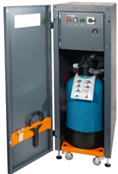
Clean as a whistle – the FilterStar and FilterStar Compact (illustrated) make dampening solution last much longer. This reduces the amount of downtime spent changing the solution and cuts disposal costs.
