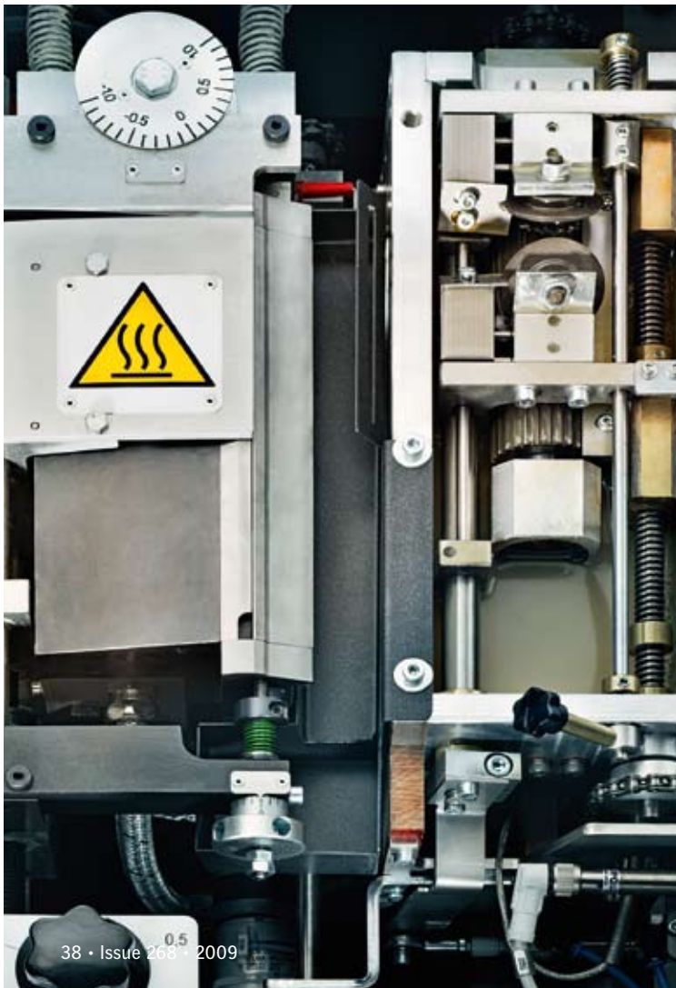
The PUR nozzle application system of the Eurobind 1300 PUR is controlled by a gear pump. As a result, it applies exactly the same amount of adhesive to each block – irrespective of viscosity, temperature or pressure (below). View of the lift-type delivery on the Eurobind 1300/1300 PUR (right).
