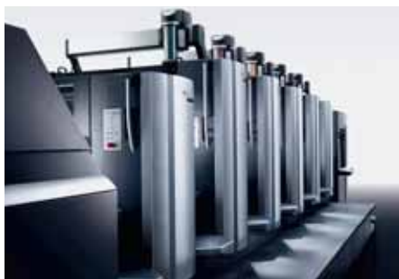
Unveiled – At IPEX in Birmingham, UK, Heidelberg premiered its new Speedmaster CX 102 which can process 16,500 sheets per hour in 27.5 by 39.3 inch (70 x 100 cm) format thanks to its XL technology.
