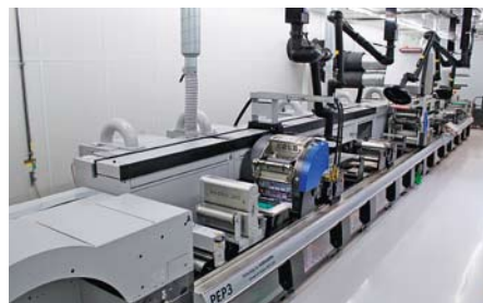
Lab press – in the near future, researchers at InnovationLab GmbH hope to print electronic circuits on film using this 17-meter long prototype from Heidelberg.
