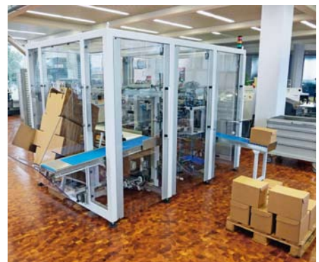
Productivity increase – the new inline case packer from Heidelberg automatically gathers and arranges product piles before packing them in corrugated cartons.
