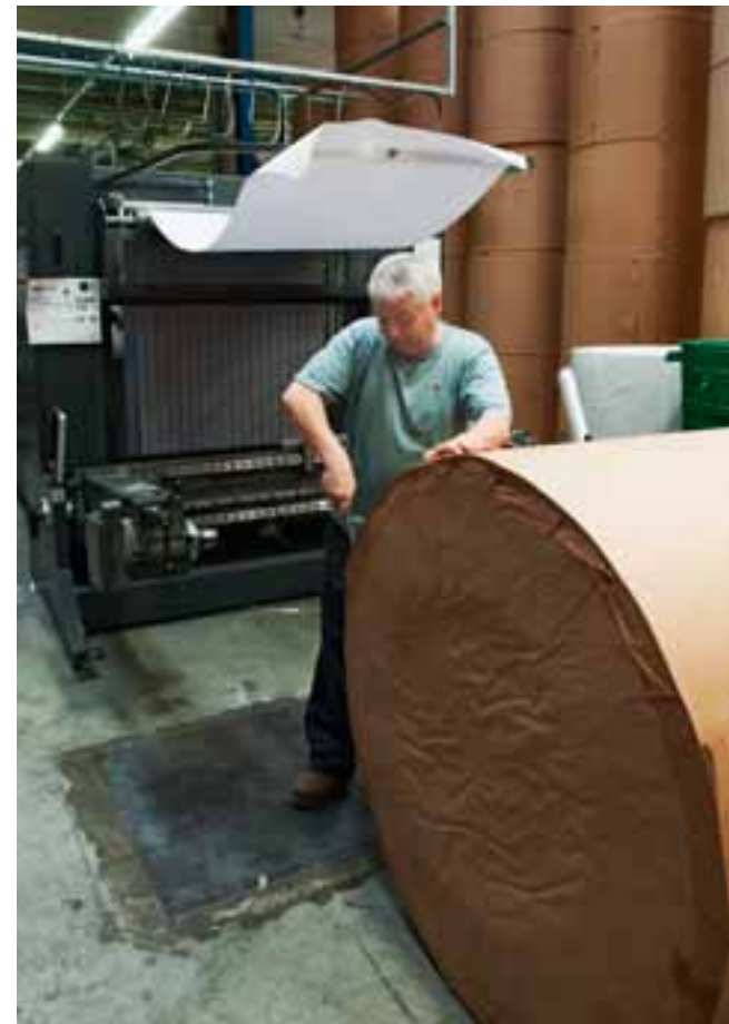
More cost-effective and up to 30 percent faster in processing – the 1.4 metric ton paper reels are moved to the press on a forklift (left) and then prepared for work with the sheeter (right).
