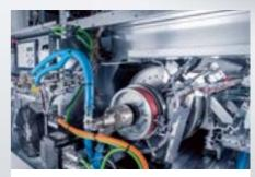
The **temperature control system** for the lasers and cylinders standardizes the imaging conditions for the plates.
