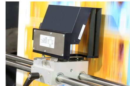
The camera-based register control uses micro dots at each station. These marks can be placed anywhere on the print image to save material. The free printing area normally reserved for the block and wedge marks becomes obsolete.
