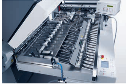
Division into two streams of sheets by the pneumatic twin-lay device.
