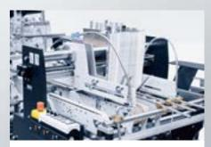
**Feeder and blank alignment** ensure precise and stable carton feeding with reliable carton alignment.
