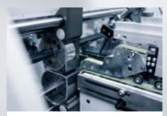
The digital position control of the Braille tools ensures precise positioning of the embossing and therefore enables production reliability.
