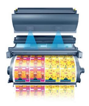
Particularly in packaging and label printing, guaranteeing the quality of a printed product is not just a matter of correct inking. Printing errors need to be identified at an early stage in order to ensure there are no complaints.
