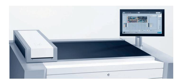
When it comes down to absolutely uniform inking over the entire sheet, you are always on the safe side with Prinect Image Control® 4. No other unit in the world spectrally scans the whole print sheet and balances out even the smallest deviations in the print image – automatically. It automatically detects not only all measuring elements but also solid areas using the prepress data and incorporates them into the control process.
