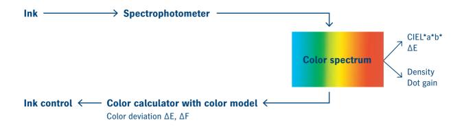
Modern color measurement systems work on the basis of a spectral photometer. These systems have the advantage of seeing more, and therefore also supply more information than traditional densito metric values CIEL\*a\*b\* and  $\Delta E$ , they also supply the density as an important control variable for the printer and the dot gain derived from it.
