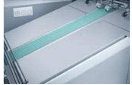
Feed table with central suction belt for precise sheet separation with a varied range of substrates.
