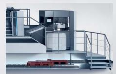
Logistics systems ensure uninterrupted non-stop production and control the automated loading of the feeder and the removal of printed pallets at the delivery.
