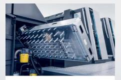
**DryStar Combination Eco** saves up to 30 percent drying energy thanks to optimized input, integrated heat recovery and insulation. It emits less heat into the workplace.
