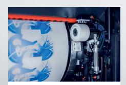
New bearer ring maintenance system and high-volume cam rollers reduce manual maintenance work and increase availability for reliable production.
