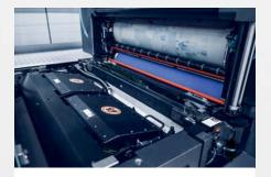
Prinect Inspection Control 4 avoids downstream costs by checking each sheet inline on each side with two highresolution color cameras for hickeys, material defects, scumming, etc.
