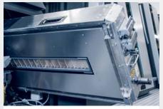
**LED dryer systems** allow direct finishing of the immediately dry sheet – a major advantage, especially for short runs and fast turnarounds.
