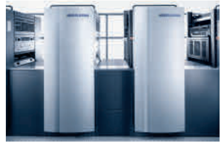
Comfortable operation thanks to freely accessible printing units and a wide gallery running along the side.
