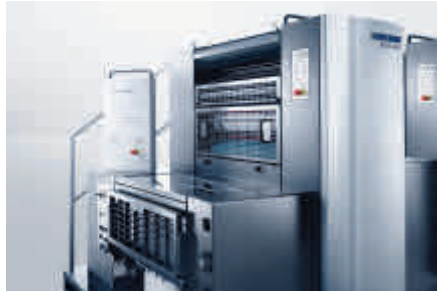
Compact standard-pile delivery with small footprint, specially designed for short and medium runs.
