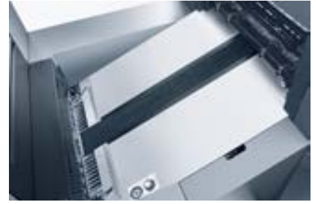
Fully automatic switchover of the Preset Plus feeder ensures the fastest material changes.
